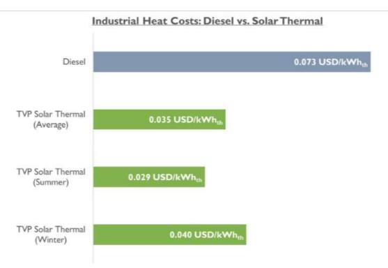
Heat prices for diesel and solar at Ocean Rubber Factory. These prices have been calculated based on a 25-year lifetime of the solar system, with average diesel boiler efficiency set to  $75\,\%$ . The cost of loans for the investment in solar was not part of the calculation.
